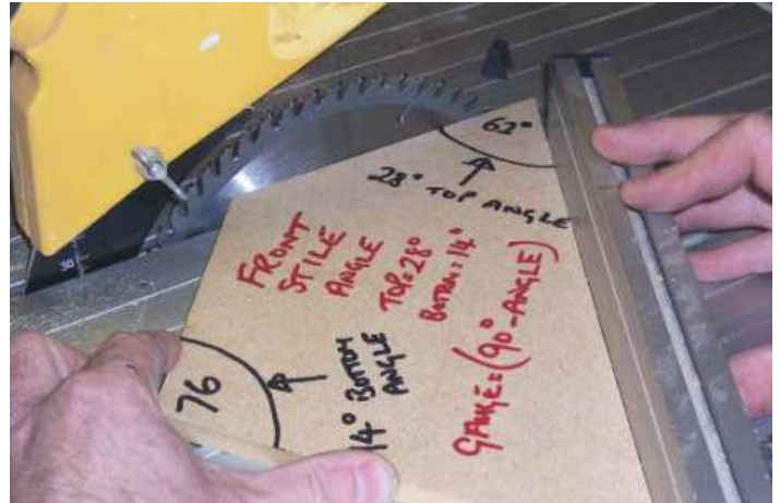
▲ Pic.2 It's a good idea to make a template for setting up the sawtable when it comes to cutting the angles for the flap
